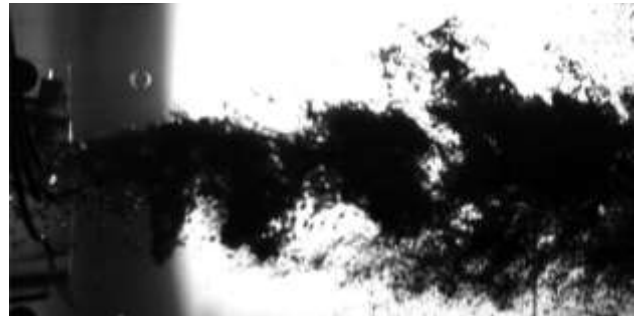
Figure 11: Visualization of the large flow structures near the exit of the half-3D divergent-convergent nozzle. Nominal void fraction at injection location was \alpha = 16\% and liquid flow rate was 0.87 \text{ m}^3/\text{min} (230 gpm).
