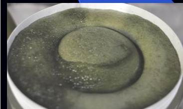
Algae floated using DYNAJETS® micro-bubble generator
