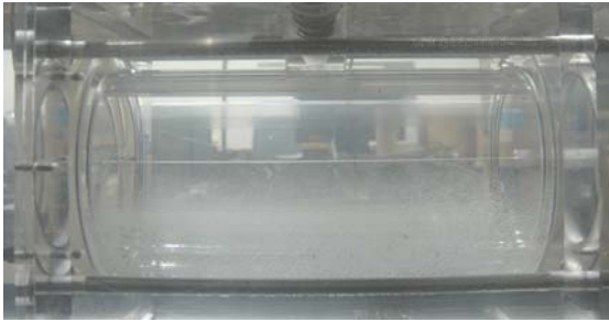
Figure 3: Picture of the vortex chamber with a cavitation core throughout.
