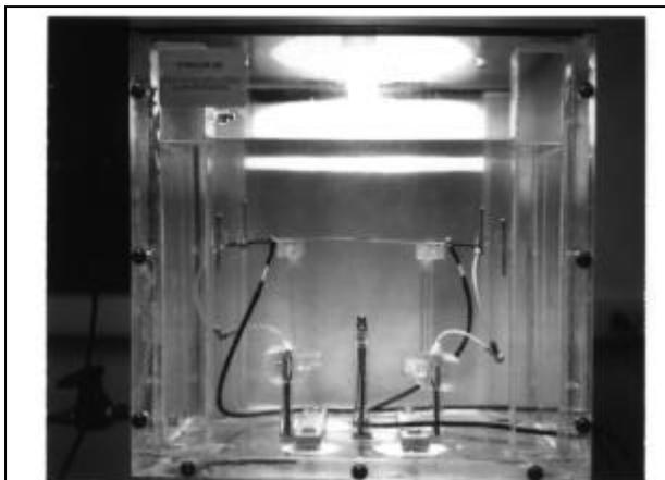
*Figure 1. Photograph of Spark Bubble Test Tank*
