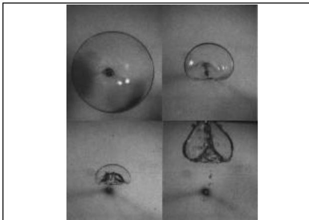
*Figure 2. Bubble dynamics in a gravity field showing reentrant jet dynamics and toroidal bubble rebound.*
