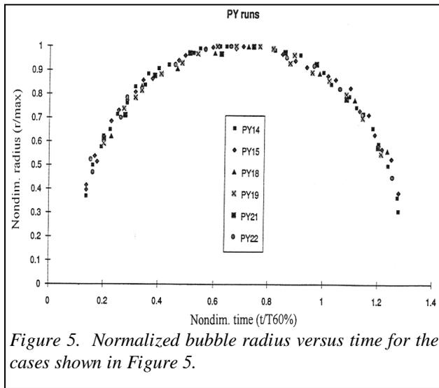
Figure 5. Normalized bubble radius versus time for the cases shown in Figure 5.
