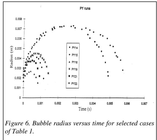
Figure 6. Bubble radius versus time for selected cases of Table 1.
